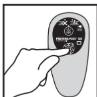
2. To begin therapy, press and hold center of the **On/Off** button for three seconds. The PREVENA PLUS™ 125 Therapy Unit, while in operation, may have a moderate sound emanating from the unit. All seven Therapy Life Indicators will illuminate with a green LED, indicating therapy is running.
