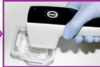
2. Attach spacer to the device
